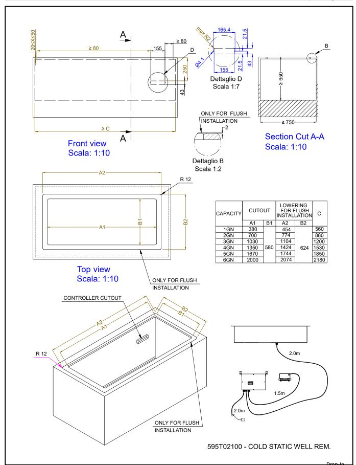
Drop-in remote refrigerated well, static (5 GN container capacity)
